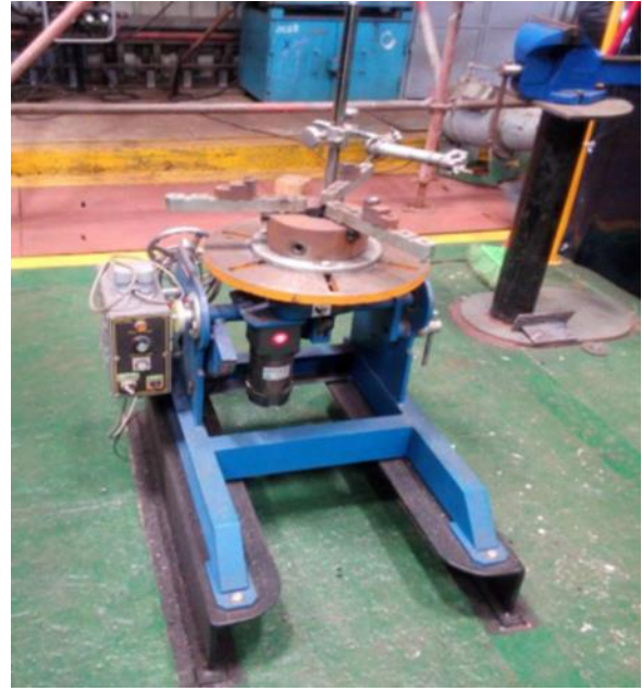
Rotating Bed for Pipe Welding
