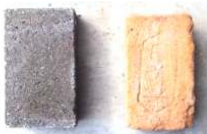
Photo: Rice husk ash brick compared to clay brick
