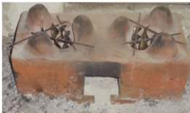
Twisted tapes sitting atop a traditional cook stove
